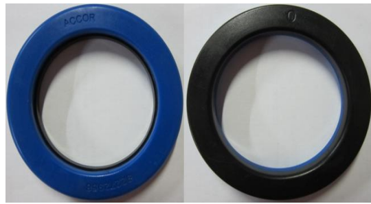
92272958 ID: 62.6mm OD: 88mm Thickness: 12mm
